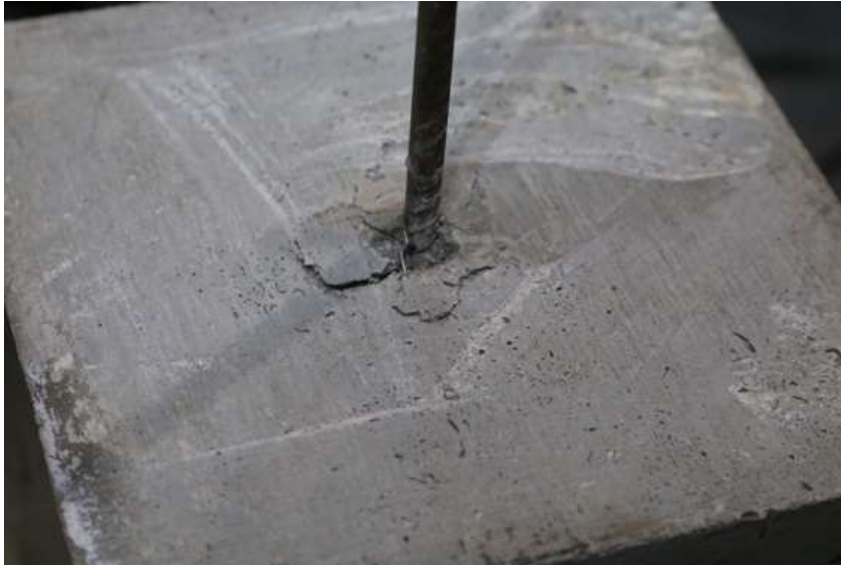
Figure 5.12 – Observed pull out failure after the mechanical test
